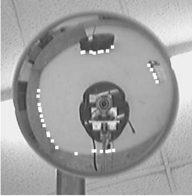
Figure 2: Leading edge detection using vision system.
